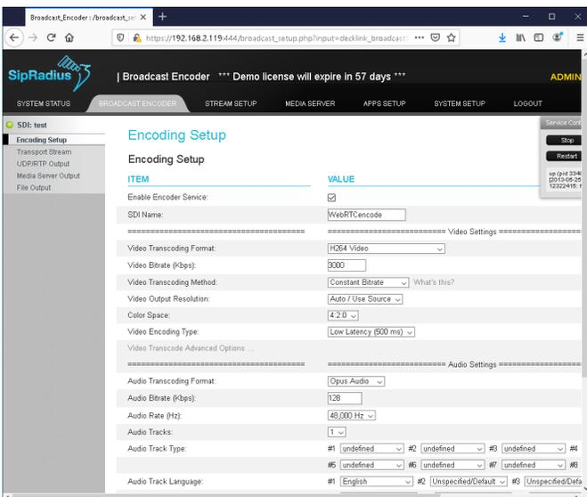
In that screen, we see low latency (ca. 500 ms, not including transit time to the end user) h.264 encoding of a 3Gbps video stream plus a 128bit opus encoded audio stream.
