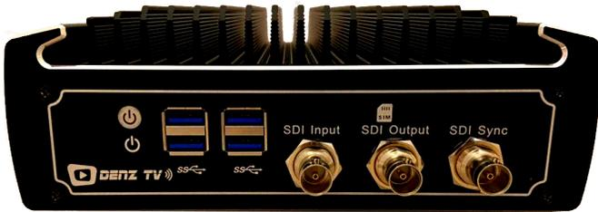
The fanless, noiseless mini PC runs our Coral OS, a customized flavor of linux designed for real-time processing and an appliance-like operation. The capture hardware will support up to 1080P/60FPS/3Gbps. The screen below shows the encoding setup:
