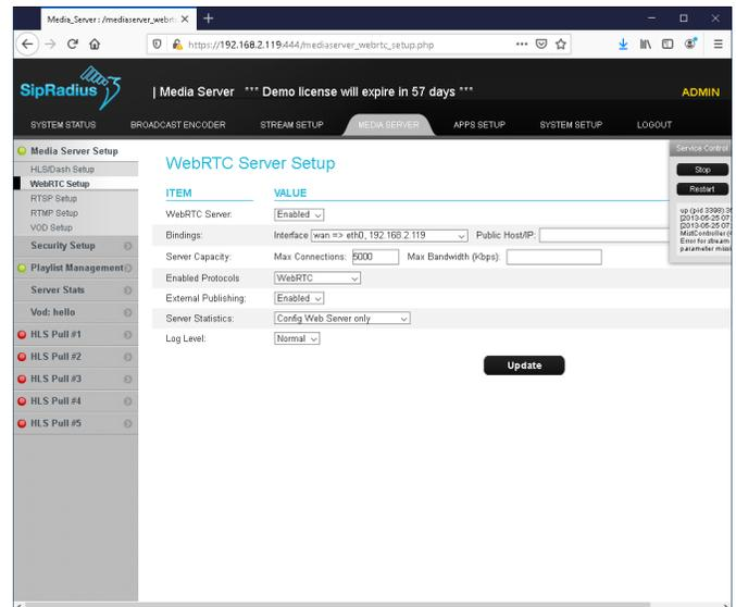
As a full featured media server, the 3G-SDI to WebRTC Server provides control over which ports to serve the output, limit the bandwidth, monitoring and statistics and so forth. There are options so that should the appliance be in a NATted private network, you can set up port
